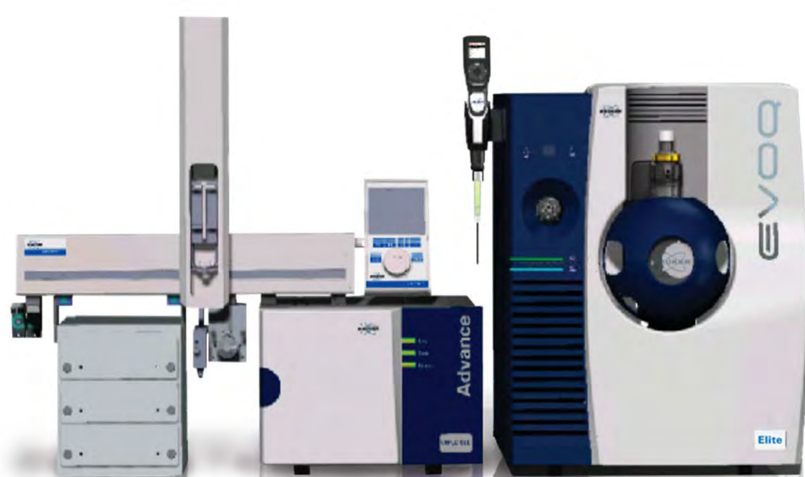
Fig. 1 EVOQ Elite triple quadrupole mass spectrometer coupled to a Bruker UHPLC and CTC Autosampler
