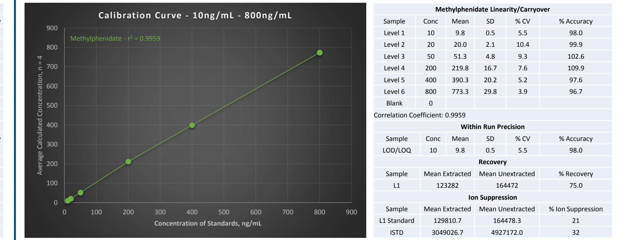
Fig. 6 Calibration curve for Methylphenidate. Correlation Coefficient is > 0.99.
