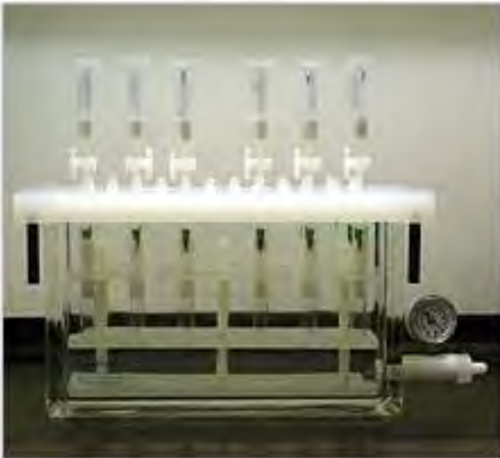
A typical solid phase extraction manifold. The cartridges drip into the chamber below, where tubes collect the effluent. A vacuum port with gauge is used to control the vacuum applied to the chamber.
