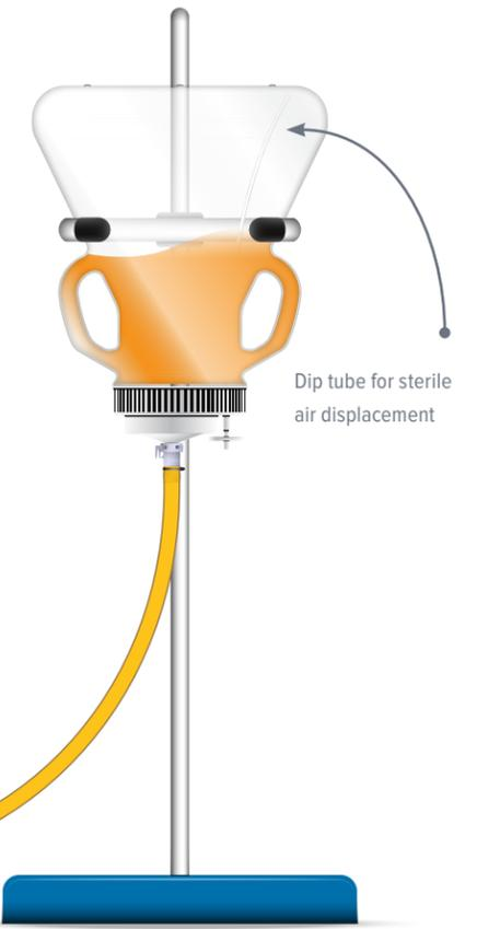
Dip tube for sterile air displacement
