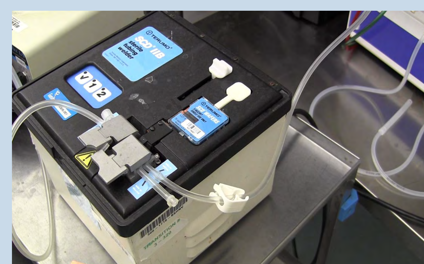
Tube fuses with C-16 C-Flex or 1/4" OD Tubing
