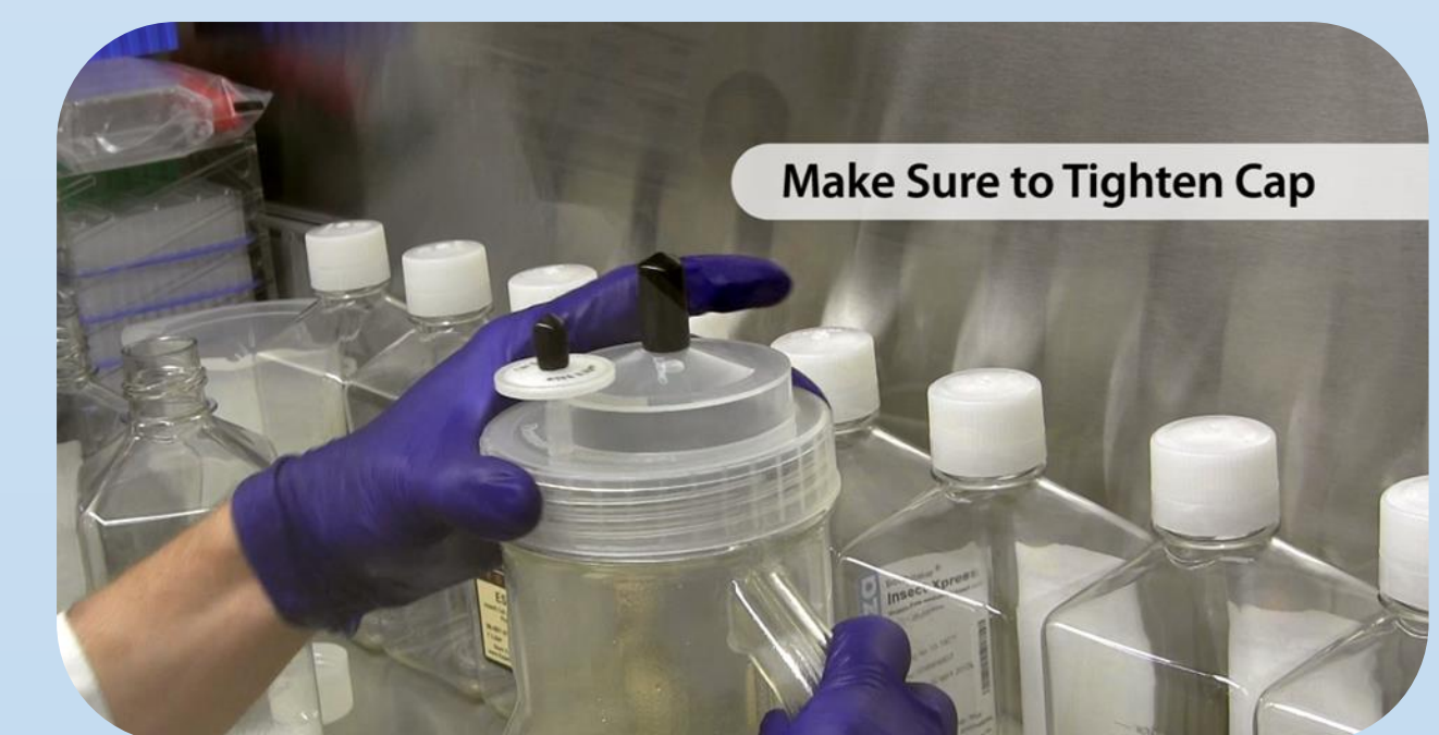
Make Sure to Tighten Cap Step 2. Check that the Transfer Cap is tight.
