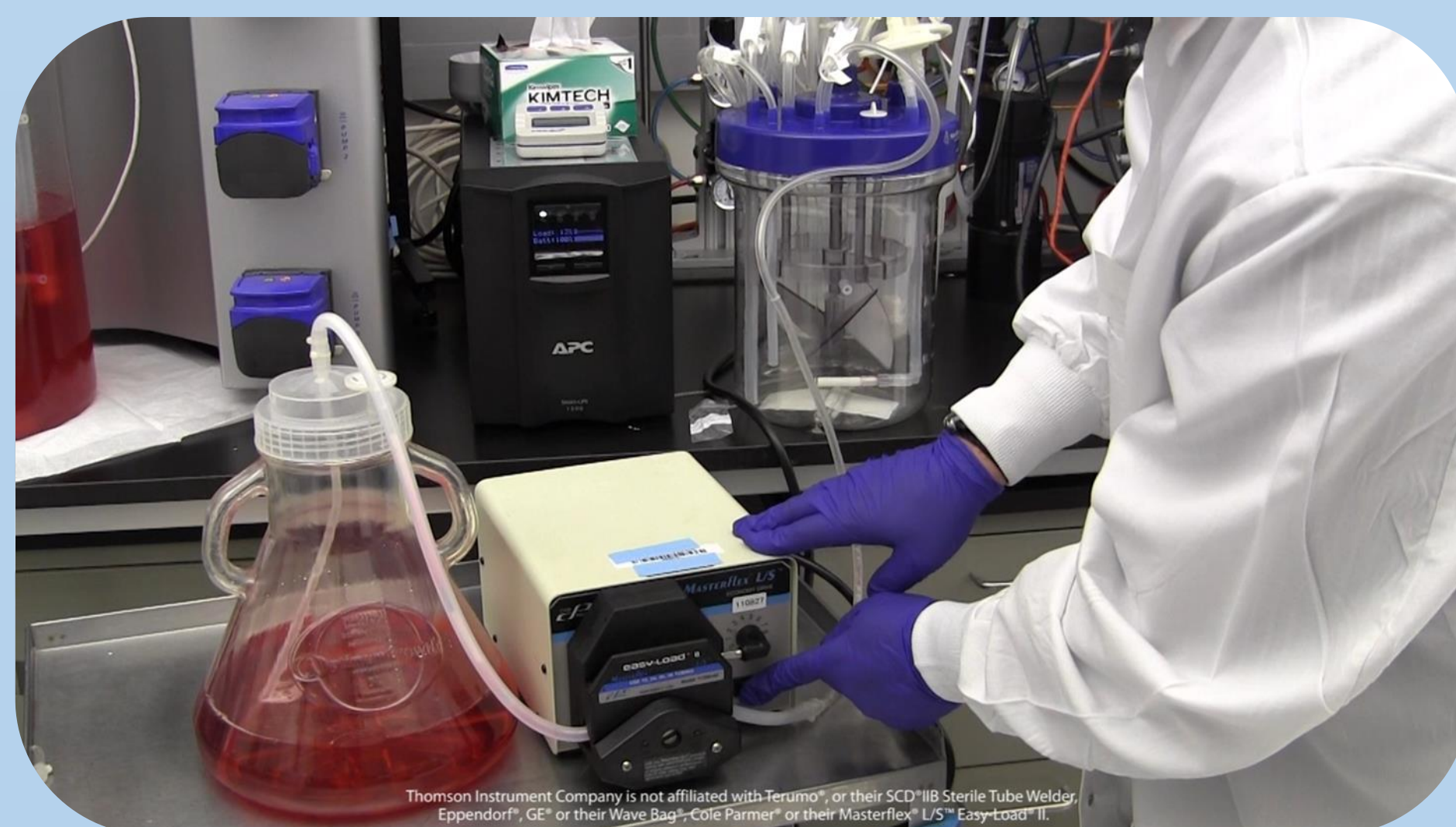
Step 5. To transfer, simply thread tubing through a pump.
