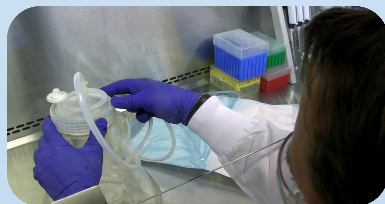
Step 2. Check that the Transfer Cap is tight.
