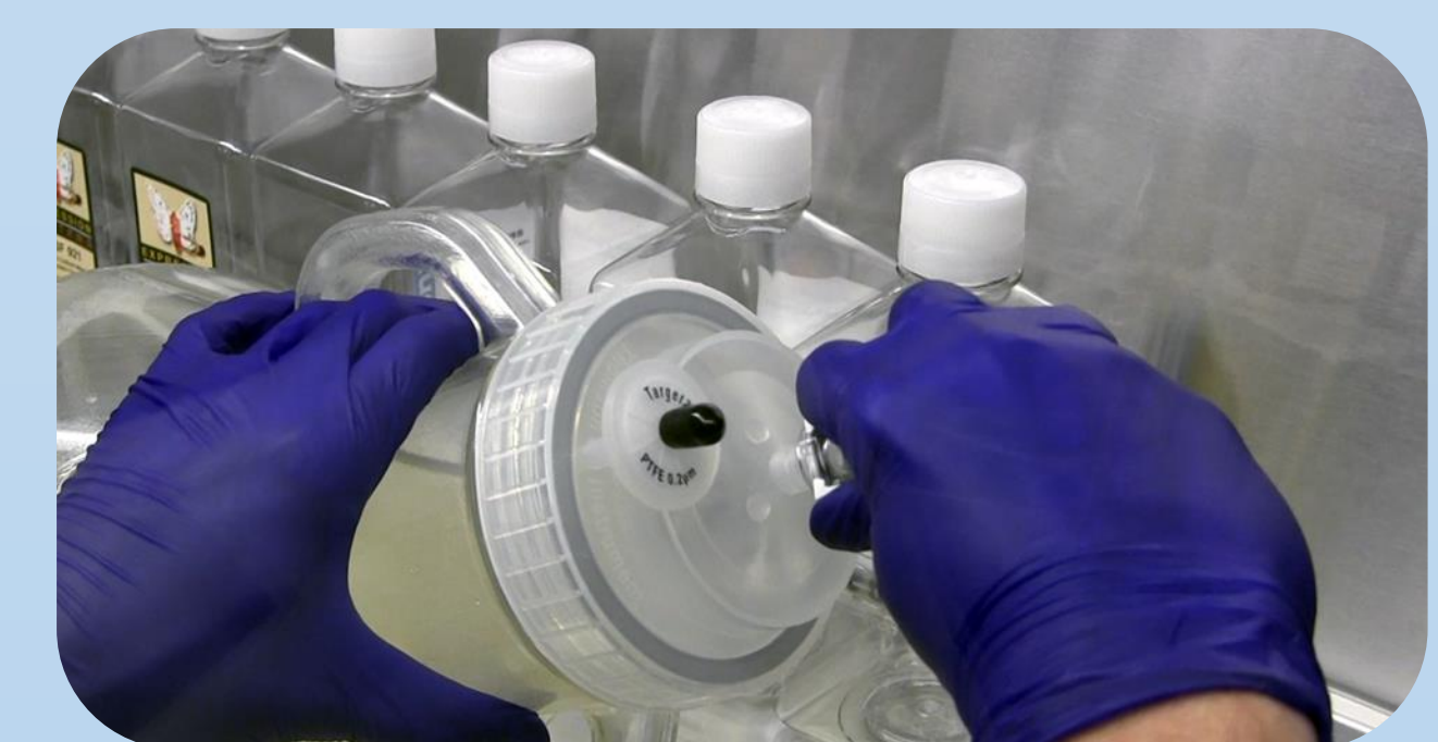
Step 3. Connect Quick Connect or Tube Fuse to Cell Bag or Bioreactor.
