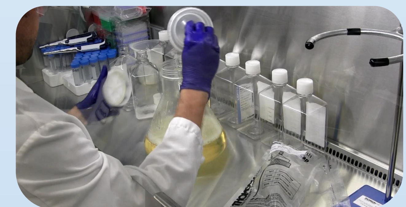
Step 1. Remove vent cap and replace with the Transfer Cap.
