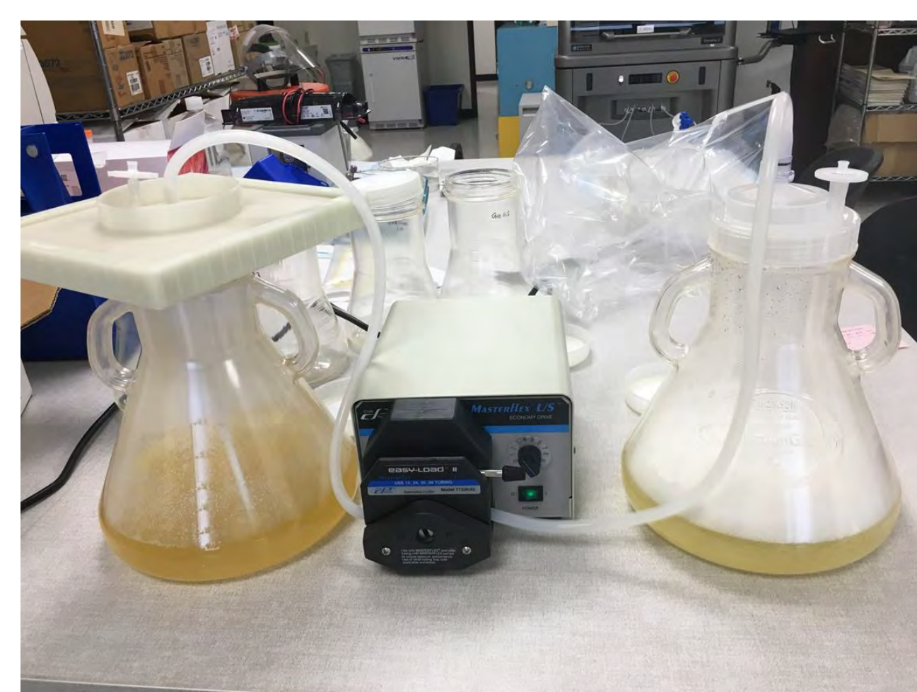
Beginning average Flow rate ~ 200ml/min Flow rates slow nearing filter capacity, average Flow Rate ~ 110ml/min
