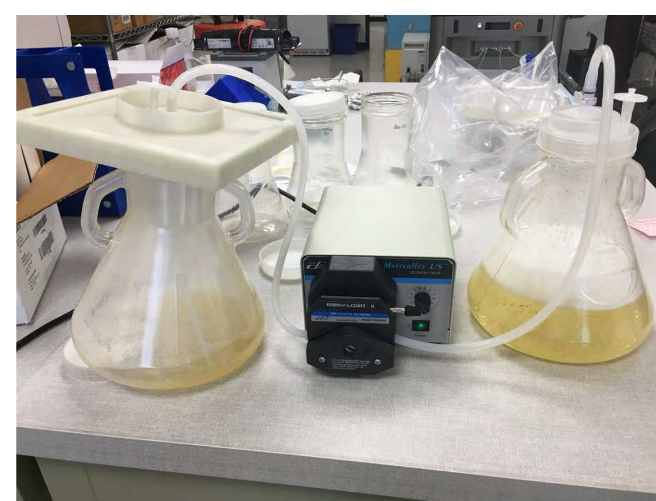
To maximize culture recovery, add 500mL of 1x PBS to the flask to flush the system at the end of filtration
