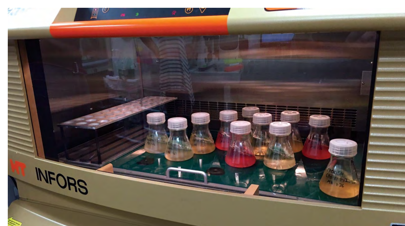
Fig 3. Optimum Growth™ 250mL Flasks in 8 Position Carrier (p/n 1212905) and in Infors Shaker
