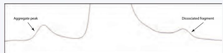
Fig 4. Zoomed in version of the chromatogram in Fig. 3 of Antibody mAb2 to better visualize aggregate peak.
