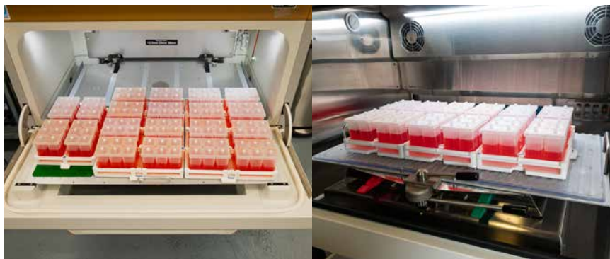
Figure 3 – 6-well plates are securely held during shaking on standard incubator/shakers. Left – Rack on Infors Shaker deck with sticky stuff (mat); Right – Rack on Kuhner deck with sticky strips.
