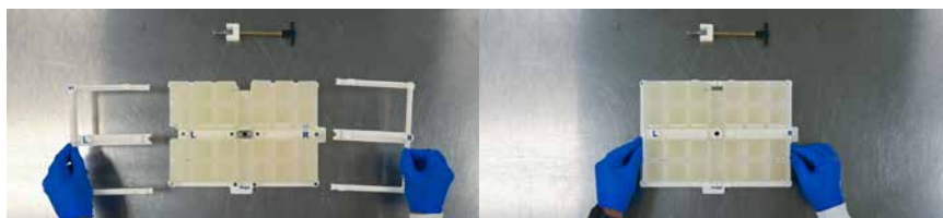
Figure 2 – Thomson 6-well culture plates are secured with the magnetic collar on the Universal 4-Position Rack for Well Plates.
