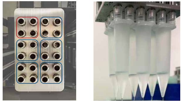
Figure 5 – Left: View of channels highlighting that one tip will engage with 4 adjacent channels on the 24-channel MCPA or ST pipetting arm; Right: Images of Mammoth 30mL Automation Tips engaged to channels.
