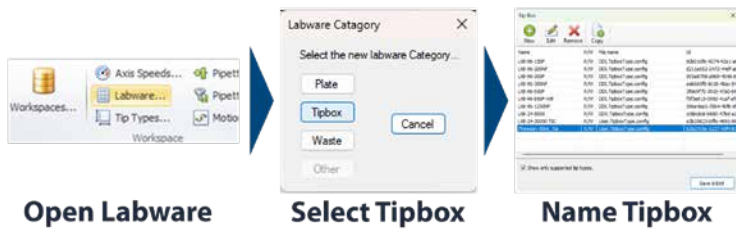
Figure 3 – Method Manager 4 software setup for Mammoth 30mL Automation Tips. Opening Labware for definitions; Selection of Tip Box; Defining Name of Tip Box “Thomson-30mL_Tip”.
