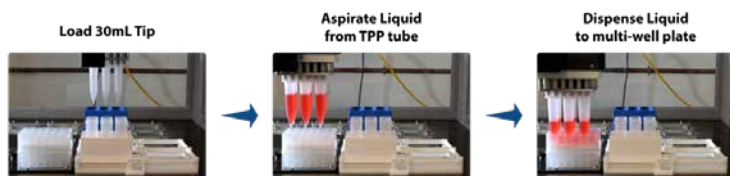
Figure 10 - Workflow of aspiration and dispensing into a Thomson 24-well plate
