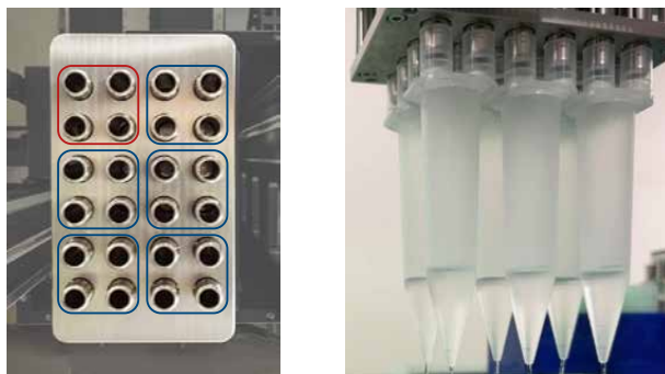
Figure 6 – Left: View of channels highlighting that one tip will engage with 4 adjacent channels on the 24-channel MCPA or ST pipetting arm; Right: Images of Mammoth 30mL Automation Tips engaged to channels.
